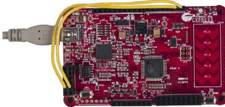
Figure 6-8. UART Connection Between PSoC 4 and PSoC 5LP
