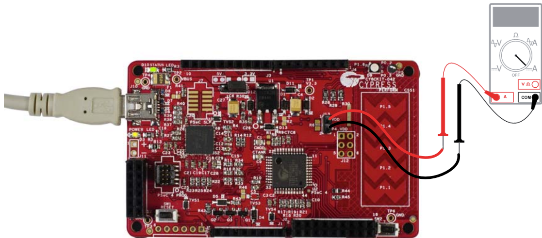
Figure 4-5. PSoC 4 Current Measurement when Powered from USB Port
