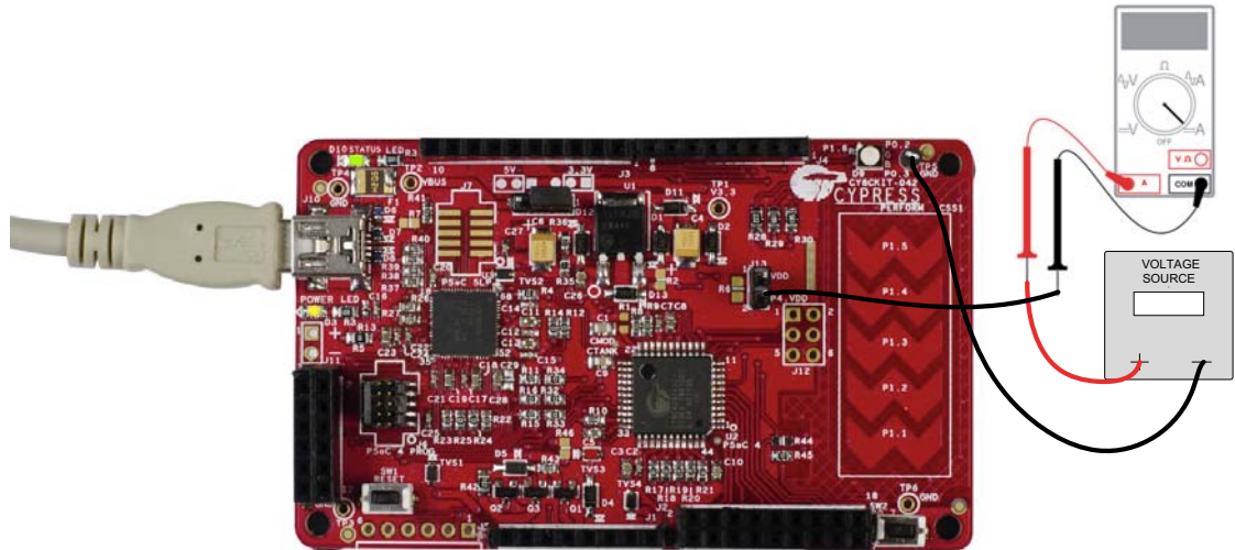
Figure 4-6. PSoC 4 Current Measurement when Powered Separately
