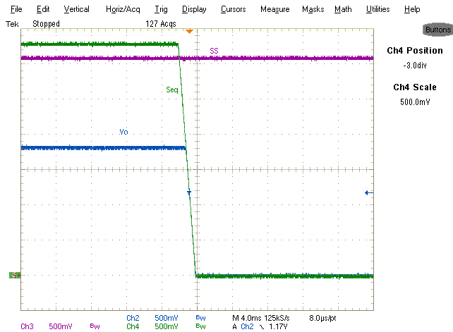
Fig. 18: Simultaneous Tracking a 3.3V input at power-up and shut-down Ch2: Vout Ch3:SS Ch4: Seq
